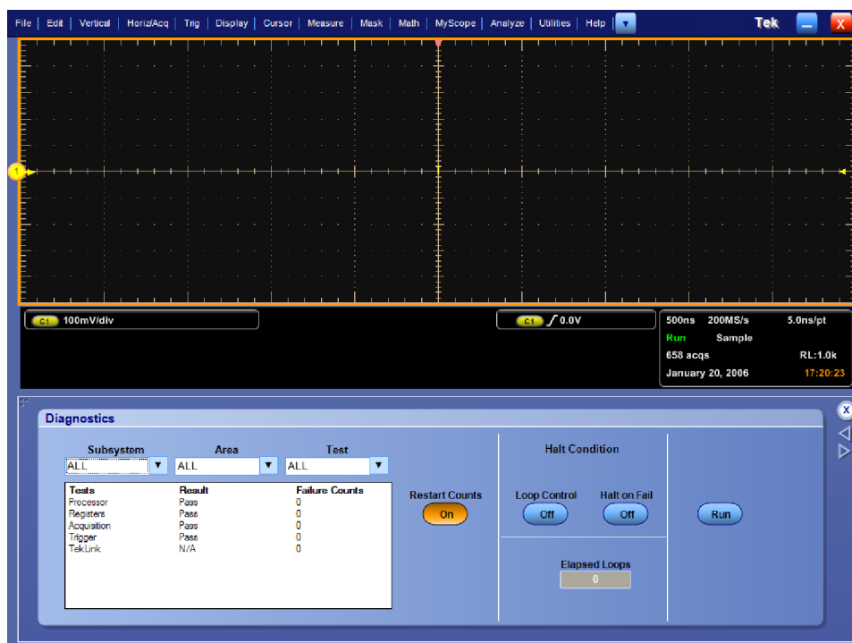
Figure 4-7: Diagnostics control panel
